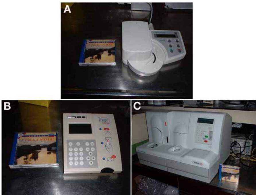
Fig. 4. Available POC instruments (the CD next to the instruments is for perspective with respect to size): (A) Cardiac Reader (Roche Diagnostics, Indianapolis); (B) Triage (Biosite, San Diego, CA); (C) Stratus CS (Dade Behring, Newark, DE).
