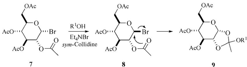
**Scheme 5.4** Orthoester formation from 1,2-*cis* acylhalogenoses.
