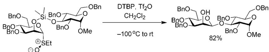
**Scheme 4.64** Sulfoxide-mediated intramolecular aglycone delivery.
