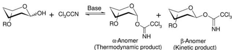
Base: NaH, Cs<sub>2</sub>CO<sub>3</sub>, K<sub>2</sub>CO<sub>3</sub>, DBU, etc.
