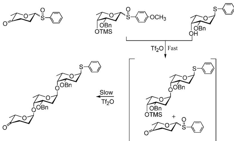
**Scheme 4.11** Chemoselective glycosidations of anomeric sulfoxides by a one-pot procedure.
