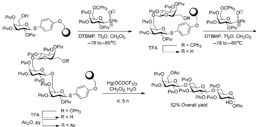
Scheme 4.67 Solid-phase oligosaccharide synthesis on a Merrifield resin.
