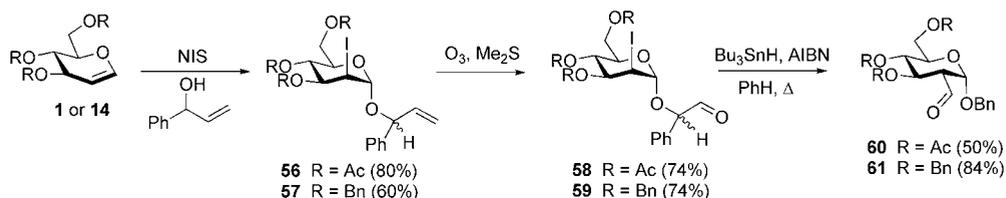
**Scheme 5.51** Method for preparation of 2-deoxy-2-C-alkylated glucosides.
