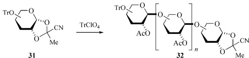
**Scheme 5.11** Polycondensation of a monosaccharide unit leading to a homopolysaccharide.
