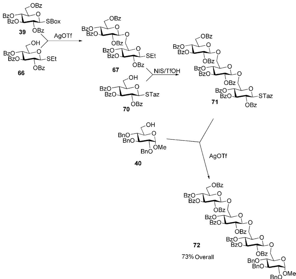
**Scheme 4.86** Orthogonal thioimidate-based, one-pot oligosaccharide synthesis [468].
