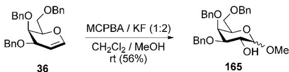
**Scheme 5.66** Use of *m*CPBA/KF in the preparation of 1,2-anhydro sugars.
