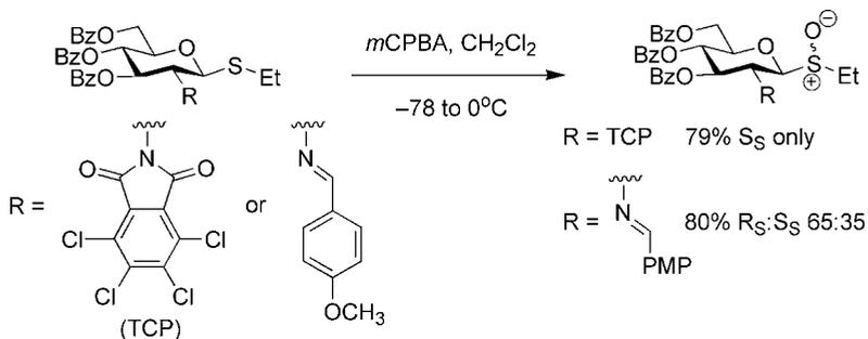
**Scheme 4.30** Protecting-group-dependent stereoselectivity in the equatorial series.
