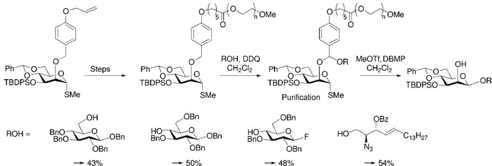
**Scheme 5.107** Polymer-supported synthesis via IAD.
