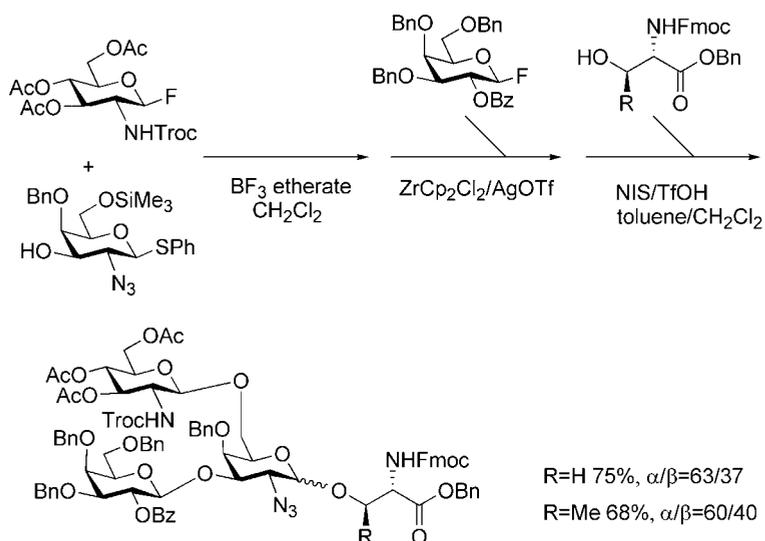
**Scheme 4.26** One-pot synthesis of core 2 class amino acids.
