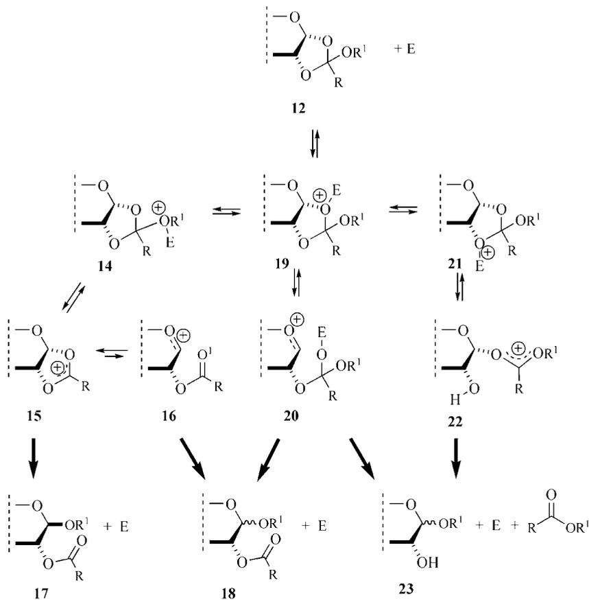
**Scheme 5.8** Proposed reaction pathways for the reaction of orthoester **12**.
