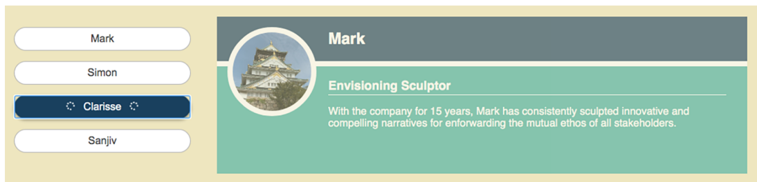
Figure 13.5 The UsersList shows the latest selection (Clarisse) with inline spinners, but the user details panel still shows the old user (Mark), the deferred value.
