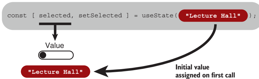
Figure 2.12 When the component first runs, React assigns the initial value you pass to useState to the selected variable.
