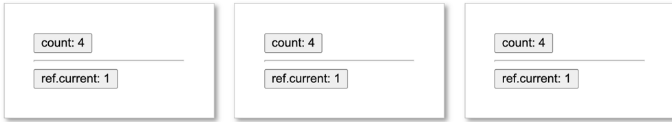
Figure 5.2 Clicking the Ref.current button three times seems to have no effect. In fact, the event handler does increment ref.current to 2, then 3, then 4, but React does not re-render the component.
