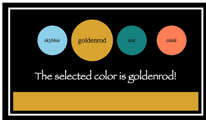
Figure 6.1 The Colors component. When a user selects a color, the menu, text, and color bar all update. When goldenrod is selected, its menu circle is larger, the text says “. . . goldenrod!” and the bar's color is goldenrod .
