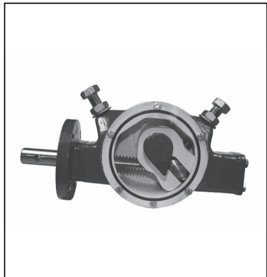
Figure 6-3 Scotch yoke traveling nut actuator cutaway
