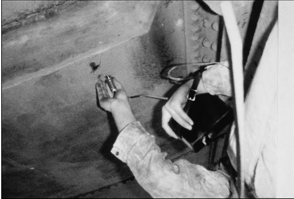
Figure 9-3 Measuring shell thickness with ultrasonic equipment
