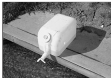
Dechlorination container is placed on the curb in a position such that the dechlorination solution will drip into the water stream.
